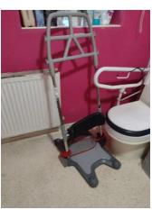
This referral was for some form of "docking" arrangement for the clients transfer appliance when she is moving from her wheelchair onto the toilet, such that it prevents the wheelchair from moving about. A retaining bracket was fabricated in steel using 40x40x03mm angle iron, which was cut to length and angled at both ends to provide a guide-in for the wheels. Once the required angle had been
