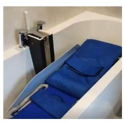
To stop this happening a removable plastic fence was made from facia panel material which fitted under the taps. and was held in place with a removeable dowel. This holds the bath guard clear of the tap spout so preventing it from getting caught when rising. The fence can be readily removed when not needed.
