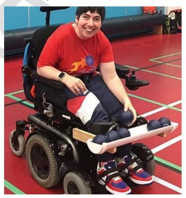
A holder made from plastic guttering was attached to her wheelchair with simple hooks. Having this equipment has placed the balls in a convenient position and made it easier for her to play.
