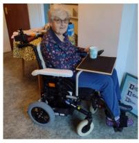
This requirement was for a swivel tray to be made and fitted to the client's powered wheelchair. She had very little use of her right side, therefore, the tray needed to be light and easy to handle with her left hand. An existing bracket on the wheelchair lower frame was utilised. A right-angled bracket
