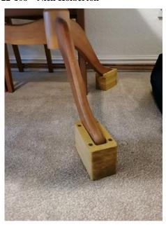
length of 35 x 70mm PAR Redwood screwed together with 70mm wood screws. The top piece had a routed recess to securely fit the leg foot. The 2nd layer had a routed space beneath and a hole drilled to allow the table foot height adjuster to screw it to the table leg foot. The 3rd and 4th layers completed the height extension. Corners were filed down and raisers were coated with satin oak furniture varnish.
