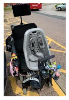
The solution to this problem used equipment designed and donated by the Leicester panel to a neighbouring few panels. The system consists of a T-bar with adjustable that fingers fit between the wheelchair seat and main cushion. The occupants weight on the cushion holds the Tbar in position.
