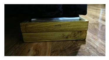
A diabetic patient required a bed raising by 2 inches. A piece of timber was cut, planed, screwed together, and routed to provide a recess. The bed legs sat inside the recesses and supported the bed safely with felt pads for protection. The outer surfaces were given 3 coats of satin medium oak furniture varnish.
