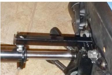
The Derby Royal Orthotics department required a standard office chair to be fitted with a device to prevent it swivelling. Mike constructed and fitted a cantilever beam to stop
