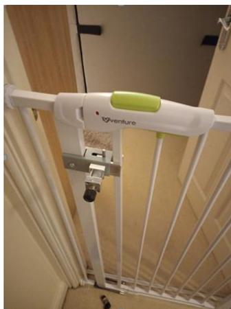
The requirement was to provide a more complex locking mechanism for a standard stair gate to prevent a boy with autism escaping from his safe area.
